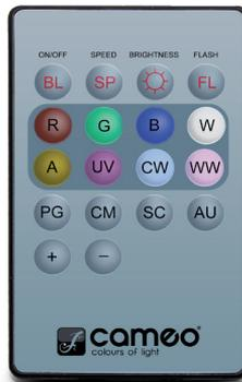
Activate infrared remote control in system settings under “IR remote” (IR Remote On). Aim the infrared remote control directly at the infrared sensor built into the front of the spotlight. The maximum range is approximately 8 metres. Deactivate infrared remote control (IR Remote Off) if you wish to control the spotlight via W-DMX.
