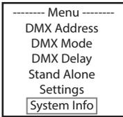
This will take you to the submenu for accessing the system information (see table, selection with UP and DOWN, confirm with ENTER, change status with UP and DOWN, confirm with ENTER).
