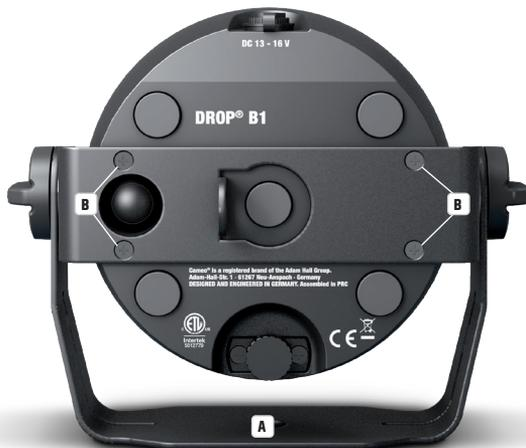
In order to effectively use the tilt function with the tilt screw when using as an uplight, and to achieve a more inconspicuous look, you must use a suitable tool to remove the mounting bracket by releasing the four T10 Torx screws (B) that secure the mounting bracket to the spotlight housing.
