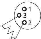
Termination reduces signal transmission problems and interference. It is always advisable to connect a DMX terminator, (resistance 120 Ohm 1/4 W) between pin 2 (DMX-) and pin 3 (DMX+) of the last fixture.
