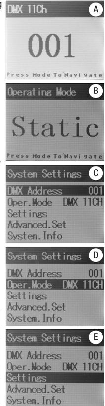
Confirm the setting changes with ENTER and press the MODE button (possibly several times) to return to the main display.
