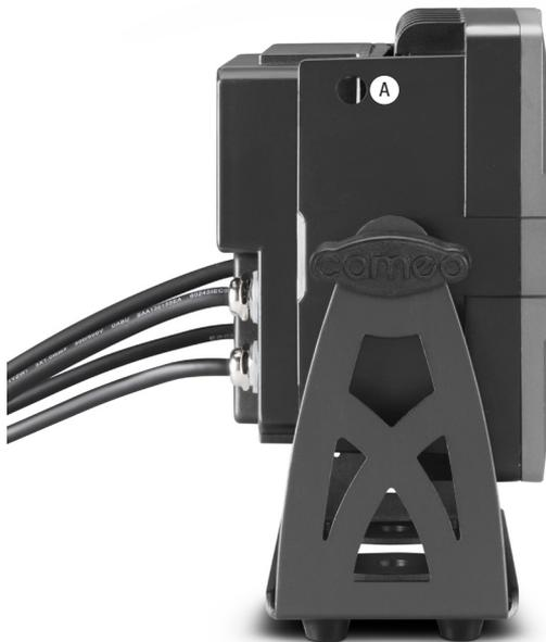
**EN** Thanks to the integrated rubber feet, the floodlight can be placed in a suitable location on a flat surface etc. Mounting on a truss is performed using a suitable truss clamp (not included) fixed to the mounting bracket; secure the device with a suitable safety rope to the chosen location (A). Important Notice: Overhead installation should only be carried out by trained personnel.
