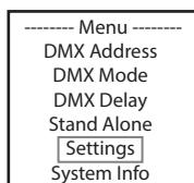
This will take you to the submenu for setting the submenu items (see table, select with UP and DOWN, confirm with ENTER, change value or status with UP and DOWN, confirm with ENTER).
