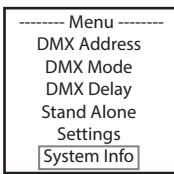
This will take you to the submenu for accessing the system information (see table, selection with UP and DOWN, confirm with ENTER, change status with UP and DOWN, confirm with ENTER).
