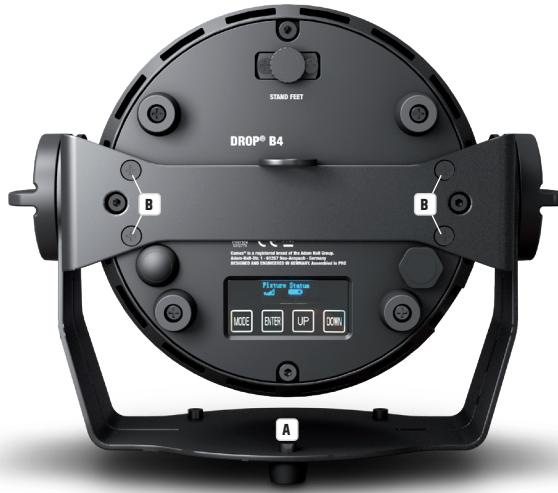
In order to effectively use the tilt function with the tilt screw when using as an uplight, and to achieve a more inconspicuous look, you must use a suitable tool to remove the mounting bracket by releasing the four T20 Torx screws (B) that secure the mounting bracket to the spotlight housing.
