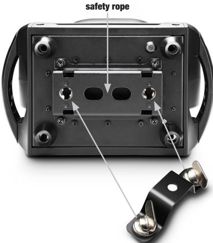
**EN** Thanks to the integrated rubber feet, the spotlight can be placed in a suitable location on the stage floor etc. Mounting on a truss is performed using the supplied omega mounting bracket (please use only the original mounting bracket); secure the device with a suitable safety rope to the space provided (please fasten the safety rope prior to installing the omega mounting bracket). Important Notice: Overhead installation should only be carried out by trained personnel.
